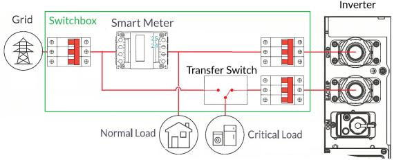
Switchbox makes the installation easier - and the power supply more reliable!
